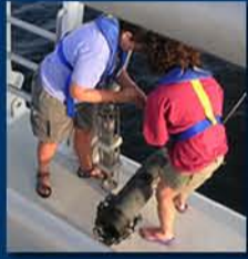
Fig. 4: The multibeam is prepared for deployment.
